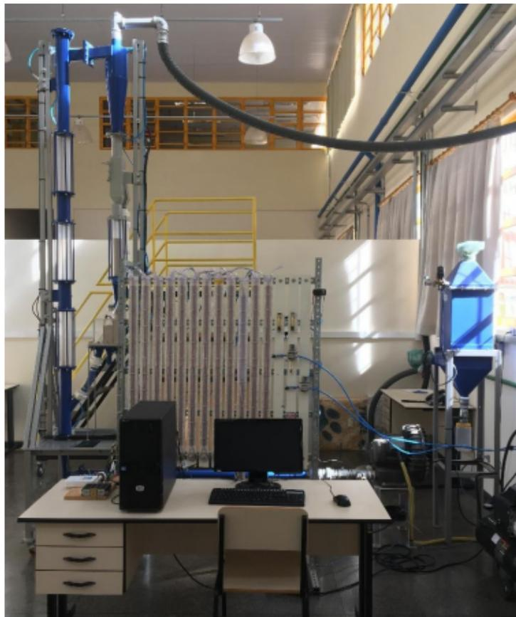
**Figure 3 – Overall view of the small CFB at the Laboratory of Thermochemical Processes - UTFPR/Ponta Grossa Campus. Source: Oliveira (2019).**
