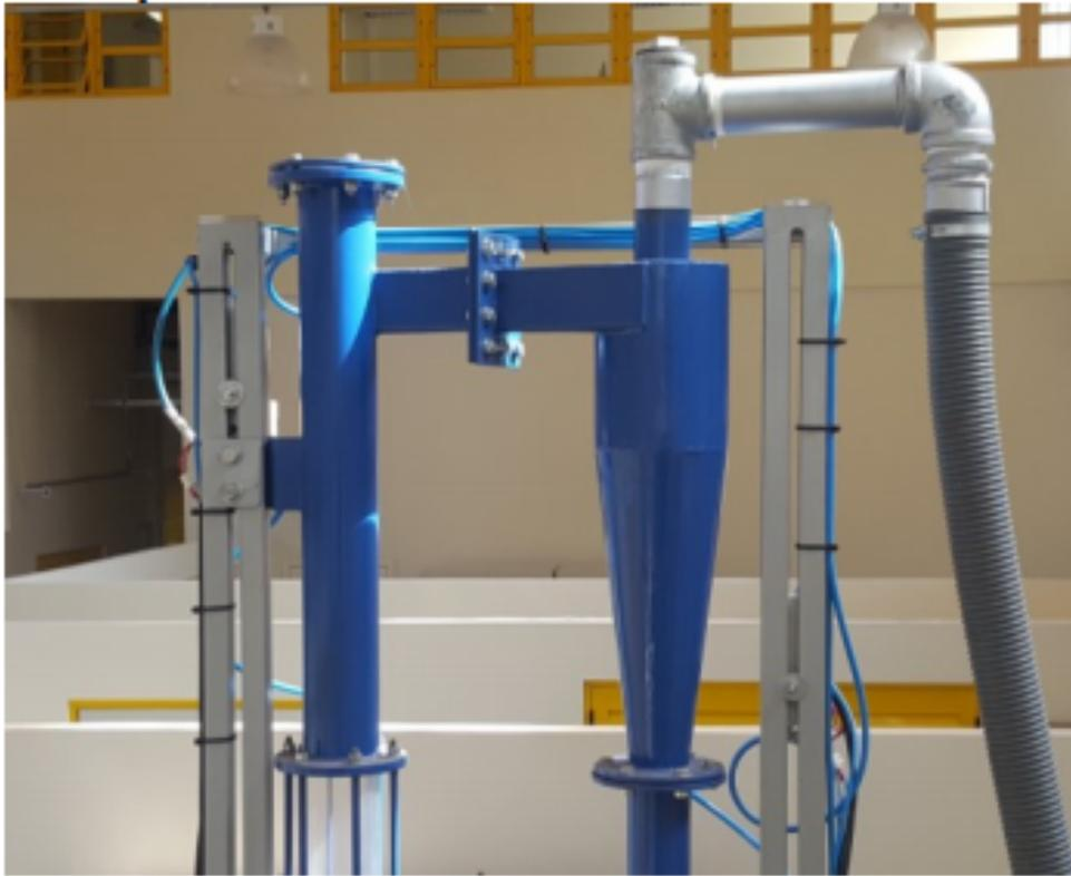
**Figure 4 – View of the cyclone coupled to the small CFB.**
